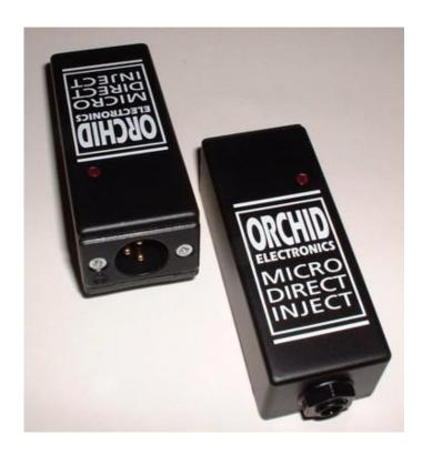
Housed in a strong aluminium die cast box 100 X 38 X 32 it has only a jack socket input for connection to the instrument and an XLR output to feed the microphone input of a mixing desk - which can be located many hundreds of metres away if necessary. It must receive Phantom Power from the mixer as it is an active design - a flush mounted red LED will indicate power present.
