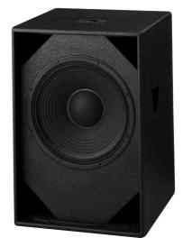
The compact Blackline \$15 sub-bass system has been designed to be used with Blackline \$12 or \$15 full-range systems to extend and increase the total low frequency output power. The \$15 provides good bass punch from a direct radiating \$15" (380mm) driver with a 4" (100mm) high temperature voice coil.
